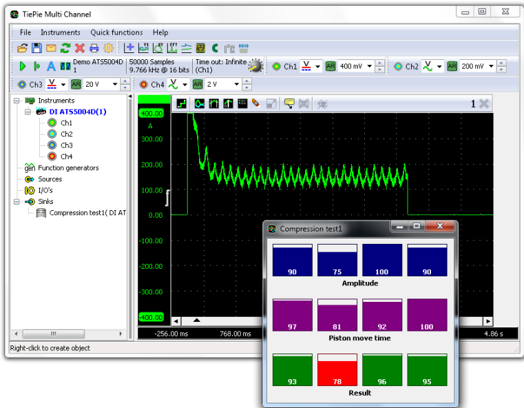
Figure 10.5: Compression test on engine with leaking cylinder
